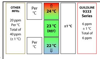
250 ppm [i.e. 50 ppm (stability) + 200 ppm (temperature affects adjustment +5 °C at 20 ppm/°C and -5 °C at 20 ppm/°C)]. Applying a general rule of 4 to 1, this allows you to calibrate only instruments with a 0.1 % or larger specification.
