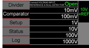
Divider. A 10 Volt Reference Standard is placed on the 7520 Reference Standard Terminals. Note that the maximum voltage that can be used as Vref is 12.5 V. The 100 V input is then divided down to equal the voltage reference of 10 V, allowing for a direction comparison of 10 Vin to 10 Vref. The voltage difference of Vin and Vref will be available at the 7520 Null Detector Terminals. Again, the divider contributes very little uncertainty to the overall measurement process.
