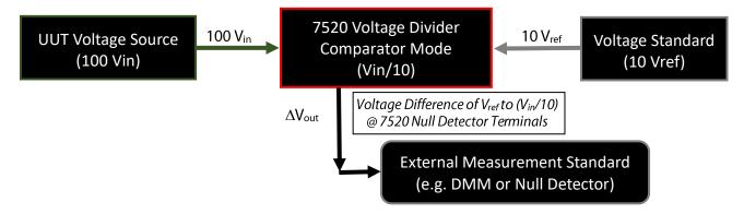
In addition, when operated in the Comparator mode of operation, the polarity of the Voltage Reference can be switched inside the 7520 manually or automatically. This enables automated polarity switching for the Voltage Reference, thus the wires connecting the Voltage reference do NOT have to be manually switched to change the polarity. This also speeds up the calibration process because there is no wait time required due to switching the Voltage Reference leads.
